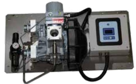
Remote mount capability enables an easier, safer means to calibrate and operate the valve
